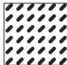
P26 Diagonal Hole Size 0.394" x 0.079" Open area 25.75% Centers 0.469"
